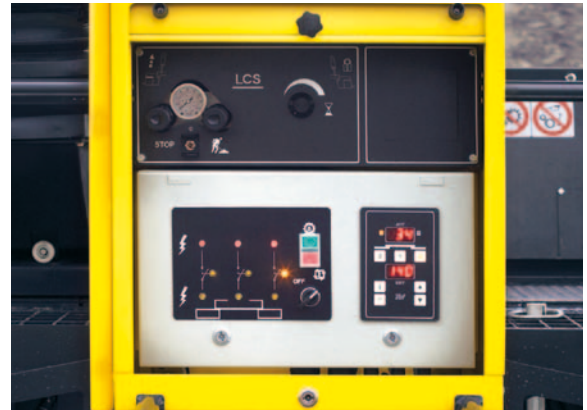
Central screed operator station
