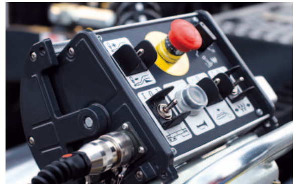
Side-mounted screed operator station
