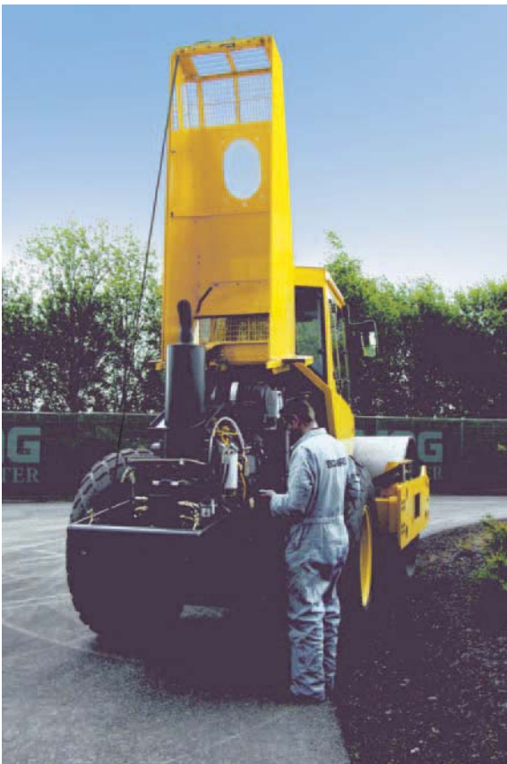
All service points accessible from the ground and hood opens manually.
