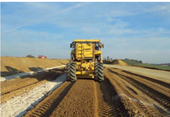
Optimum mixing quality and uniform layer thickness with BOMAG FLEXMIX technology.
