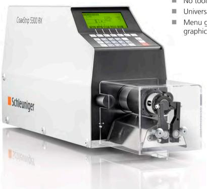
The CoaxStrip 5300 RX quickly and accurately strips wires and cables that would be virtually impossible to strip by hand. The CoaxStrip 5300 RX strips extremely thin micro-coaxial cables down to inner diameters of only 0.07 mm (42 AWG) at short cycle times. Its high-speed rotary stripping head guarantees maximum precision and prevents maintenance-related machine downtime.
