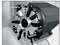
Both ST-10 models are equipped with a 12-station turret (BOT or hybrid BOT/VDI) that indexes quickly to reduce cycle times.
