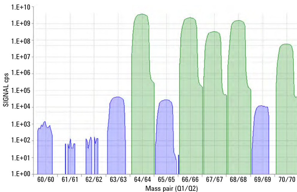
Figure 3. 1000 mg/L Zn spiked with 1 \mu\text{g/L} Cu. (1 ppb: 63/total = 0.667, 65/total = 0.333, no mass bias correction performed. If there was some contribution from Zn it would influence m/z 63 differently from m/z 65, because of the different abundance of the Zn isotopes).
