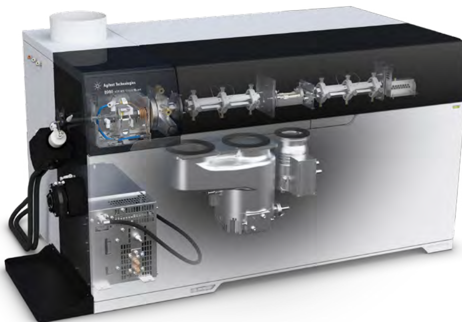
Figure 1. Cutaway diagram of the Agilent 8900 ICP-QQQ
