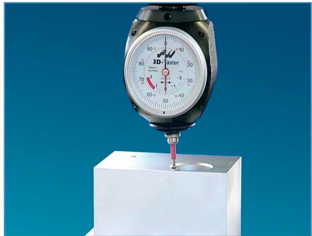
Orientate the machine spindle with the center of a drilled hole or cylindrical O.D.
