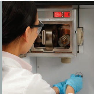
2) Rotate load coil into desired horizontal orientation
