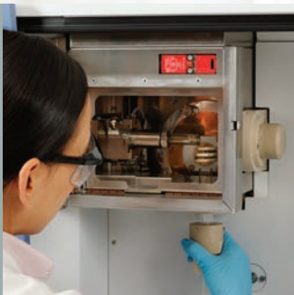
1) Simply remove radial torch and interface
