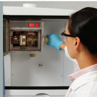
3) Install axial torch and interface
