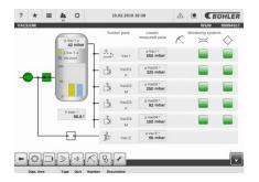
Integrated seamlessly into your Fusion machine, the SmartVac vacuum system is controlled centrally from the DataView control unit. The activation of vacuum valves is programmed according to certain machine movements. All relevant vacuum parameters are measured, monitored and assigned to the process directly – giving you comprehensive process transparency and optimum quality in the components you are producing.
