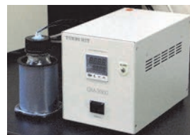
CO 2 gas injection unit
