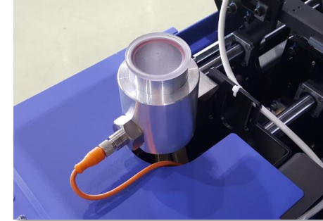
CHAIN OIL LEVEL ALARM
