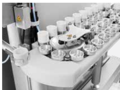
Sample feeding with the Autoloader
