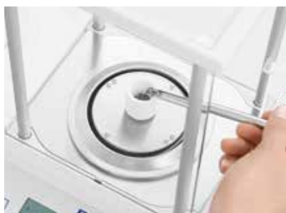
Weighing in the sample
