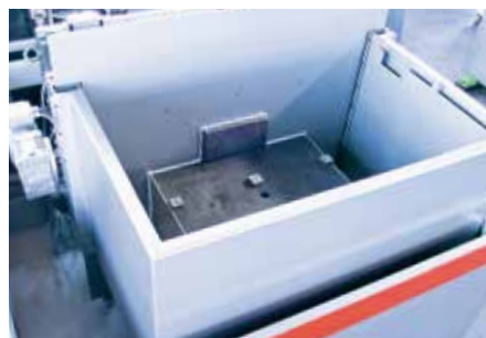
Dielectric tank Low-maintenance due to seal-free design
