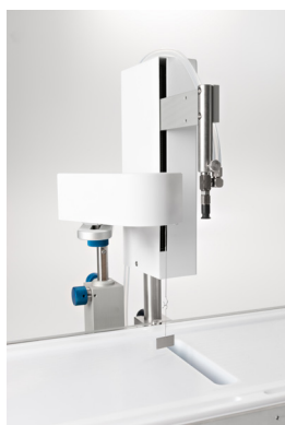
Figure 2 Langmuir and Langmuir-Blodgett trough (above) and Langmuir-Schaeffer holder (below to the left) and MicroBAM (below to the right).
