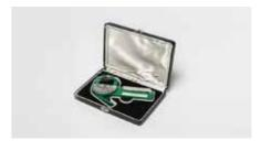
«LANGE» Skinfold caliper (made in USA) to assess Skull bowl for cubic craniophor degree of fatness Measuring range: 0 - 60 mm
