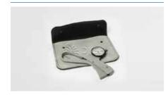
«GPM» Skinfold Caliper (made in CH) to assess the degree of fatness Measuring range: 0 - 45 mm
