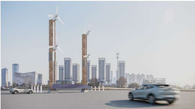
FlowGen microgrid with 4 wind turbines on 2 laminated wood masts, solar panels and battery
