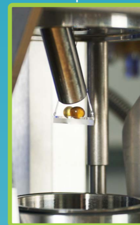
Raman probe observing samples during measurements
