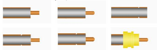
Remark: To prevent damage to the dielectric, the outer conductor is partially turned down, leaving a small web of uncut material. A hand tool supplied with the machine is used to sever the remaining material and the outer conductor will slide off easily.
