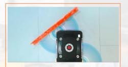
L1000 is equipped with dual LiDAR scanners with 360° coverage to support multiple levels of operational safety and security. They are the pillars to ensure a safe and reliable autonomous operation all year long.
