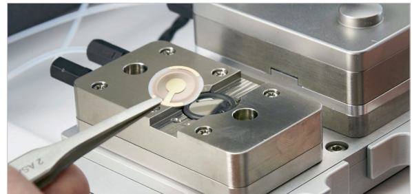
Temperature controlled environment for sensor and sample
