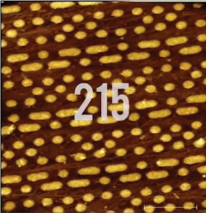
AFM topography scans of an Intel microchip (copper on silicon dioxide). Number indicates scan number as part of a time lapse of scans. Image quality (lateral resolution) does not degrade after over 1000 scans.
