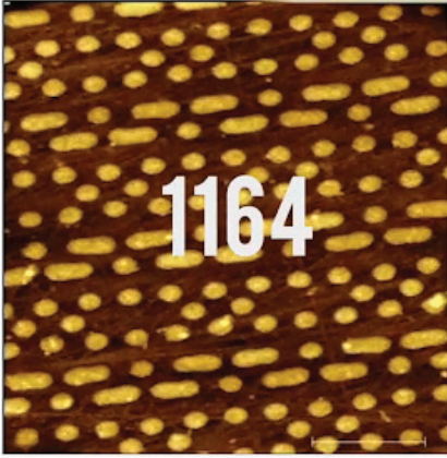
AFM topography scans of an Intel microchip (copper on silicon dioxide). Number indicates scan number as part of a time lapse of scans. Image quality (lateral resolution) does not degrade after over 1000 scans.
