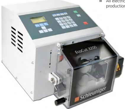
The EcoCut 3200 is an automatic cutting machine for measuring and cutting round material and tubing. The double stroke cutting head achieves a very high production rate for high efficiency while maintaining outstanding quality. The EcoCut 3200 features several interfaces for peripheral components.
