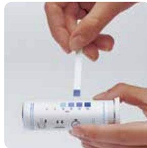
After the specified reaction time (maximum one minute), compare the color of the reaction zone with the color scale printed on the tube label to determine the concentration.
