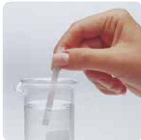
Dip strip into the test solution to wet reaction zones. Remove excess liquid by shaking test strip or drawing it across the edge of the vessel.
