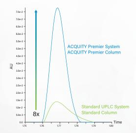
Analysis of dexamethasone sodium phosphate. Significant peak area improvement and reduced peak tailing demonstrated with ACQUITY Premier Solution compared to conventional LC technology.
