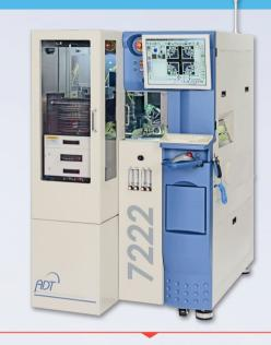
The 7200 system offers a wide range of advanced automation and process monitoring option to meet the throughput and quality requirements of your most challenging dicing applications: silicon, glass on silicon, glass, BGA & QFN packages, LTCC, ceramic, PCB and other hard material applications.
