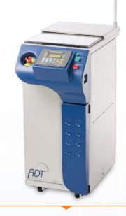
Designed for after-dicing workpiece cleaning and drying. Equipped with a spinning chuck table and a rotating washing/drying arm. The arm can be configured with an atomizing cleaning nozzle or a high pressure nozzle to cope with a wide range of cleanliness requirements.
