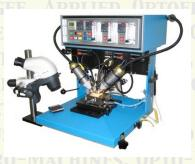
HGRS HOT Gas Workstations safely remove components from assembled circuits with momentary jets of precisely localized very hot Nitrogen. A full suite of tools also make these machines the ideal "thermal workbench" for prototypes & advanced applications.
