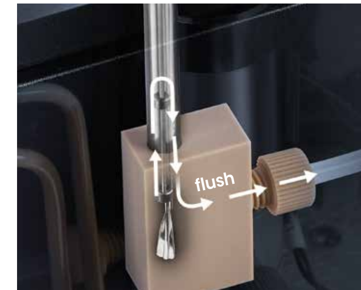
Dedicated Wash Station
