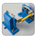
required to break the specimen and the subsequent impact strength calculated. Complies to International Test Standards ISO 179, ASTM D256, ASTM D6110, DIN 53453, DIN 53753, and BS 7413. Impact hammer energies are available from 0.5 J up to 50 J
