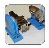
tubing for impact strength properties as either complete segments or small sections of pipes. Sample diameter dimensions up to 25 mm can be tested with hammer energies of 7.5 - 15 J. The test specimen is supported as a horizontal
