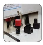
If a particular component has a critical cross sectional area that needs to be tested then by entering this area into the microprocessor the energy in KJ/M<sup>2</sup> can be obtained.
