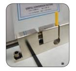
to break the specimen and the subsequent impact strength calculated. Notched or Un-notched specimens can be tested using the Izod method. Complies to International Test Standards ASTM D256, ASTM D4812 and ISO 180. Impact hammer energies are available from 0.5 J up to 25 J
