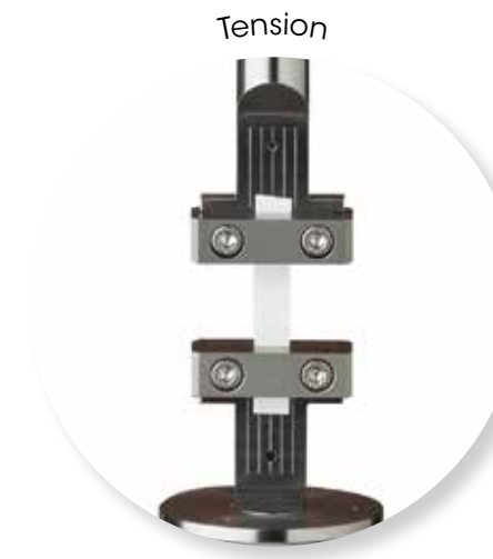
PET Film - Tension 50 μm thick
