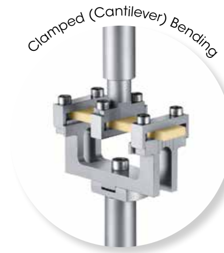
ABS bar - Cantilever 3 mm x 12.75 mm x 25 mm
