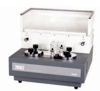
Systech Illinois' 7002 Water Vapor Transmission Analyzer delivers the same high performance as the 7001 but with an extended measurement range for more demanding applications.
