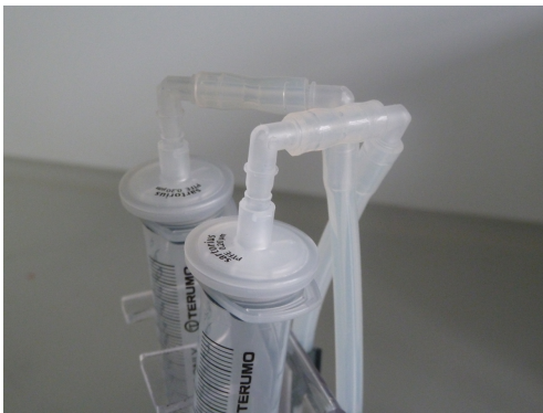
Figure 57 – Cross the tubing on top of the reservoirs to test if the problem is with the Perfusion Set or in the valve block (valve 1).
