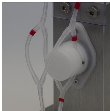
Figure 23 – Insert the tubing coming from reservoir B into the right side slots. The marked tubing goes in the rear slot.
