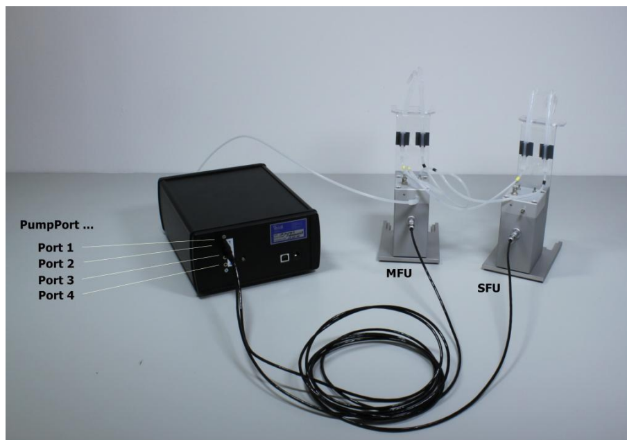
Figure 42 – Oscillatory flow setup with two Fluidic Units (one main and one secondary).
