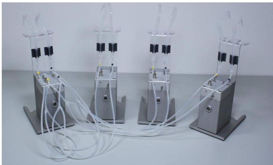
Figure 44 – Oscillatory flow setup with four Fluidic Units (one main and three secondaries).
