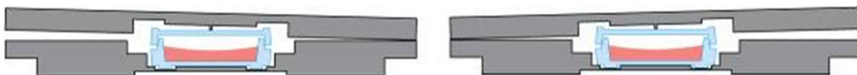
Figure 10 – Schematic Drawing of \mu -Dish in the Heating Insert. To ensure a tight fit, the lid of the Insert is tilted when closed.
