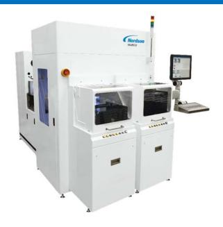
Production-ready end-effectors support vacuum, backside or edge-grip transfer. End effectors connect to a dual-arm, 3-axis transversal robot for efficient substrate handling.
