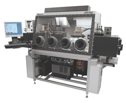
AX5000 is an ideal glovebox for the precise control of moisture, pressure and gas composition of a processing environment. It provides fully-integrated computer control of the system including enclosure pressure, interior and exterior doors, gas and moisture analysis and control instrumentation, vacuum ovens, and antechambers. The glovebox can maintain an inert environment with ultra-low moisture and oxygen levels to meet the most demanding process standards.
