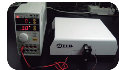
④ Press RUN button of the power supply equipment and start blotting.
