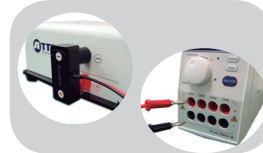
③ Set the upper electrode on the lower and connect power supply equipment with lead wire.
