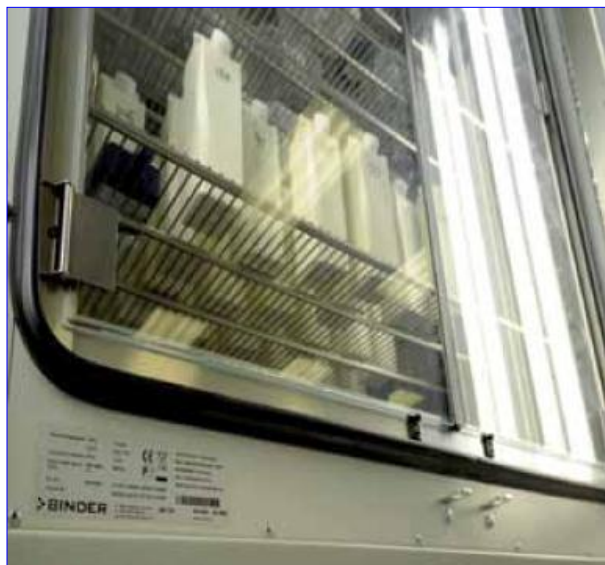
Figure 1: Constant climate chamber (Binder KBF 720) with door mounted lights used at Leatherhead Food Research for colour stability testing. 3
