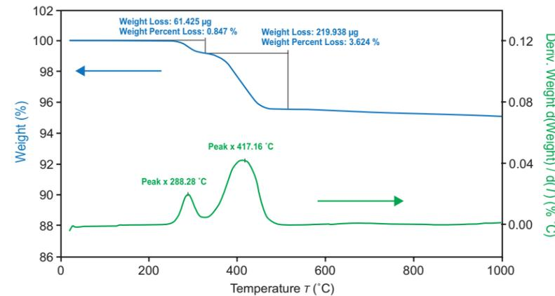
**Figure 2.** TGA curve of graphite anode in a TA Instruments Discovery TGA. The sample was heated to 1000 °C at 10 °C/min under inert conditions. The graphite anode materials contained CMC and SBR as binder and additive respectively. Thermogravimetric analysis shows that the graphite anode material was stable until approximately 288 and 417 °C resulting in small weight percent losses of 0.8% and 3.6%, respectively related to the CMC and SBR content.
