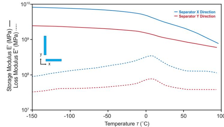
Figure 7. DMA of separator film in x- (blue) and y- (red) direction. The storage ( $E'$ ) and loss ( $E''$ ) moduli of the material are significantly different when measured along different directions.
