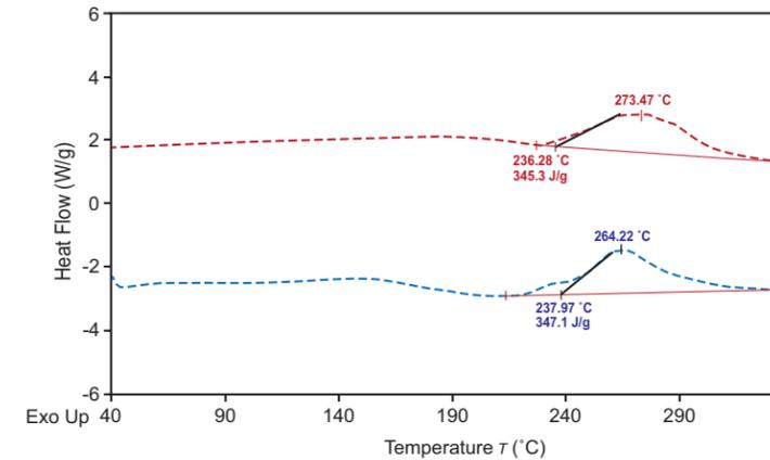
**Figure 4.** DSC curve of electrolyte measuring the onset, peak temperature, and heat of reaction during exothermic decomposition, or equivalently thermal runaway reaction. The onset temperature indicated the temperature runaway start, and the heat of reaction indicated the total heat release during the runaway reaction, which are two important parameters for battery safety evaluation.
