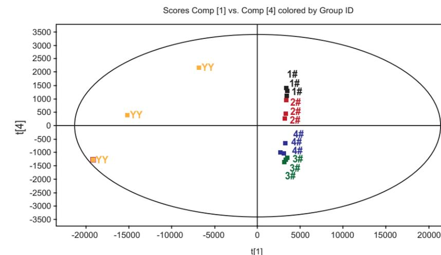
**Figure 11.** Principal component analysis (PCA) results comparing an electrolyte solution prior to the discharge-cycle (YY) to triplicate analyses of the samples that underwent 1, 40, 180 and 200 charge cycles (1#, 2#, 3#, 4#).
