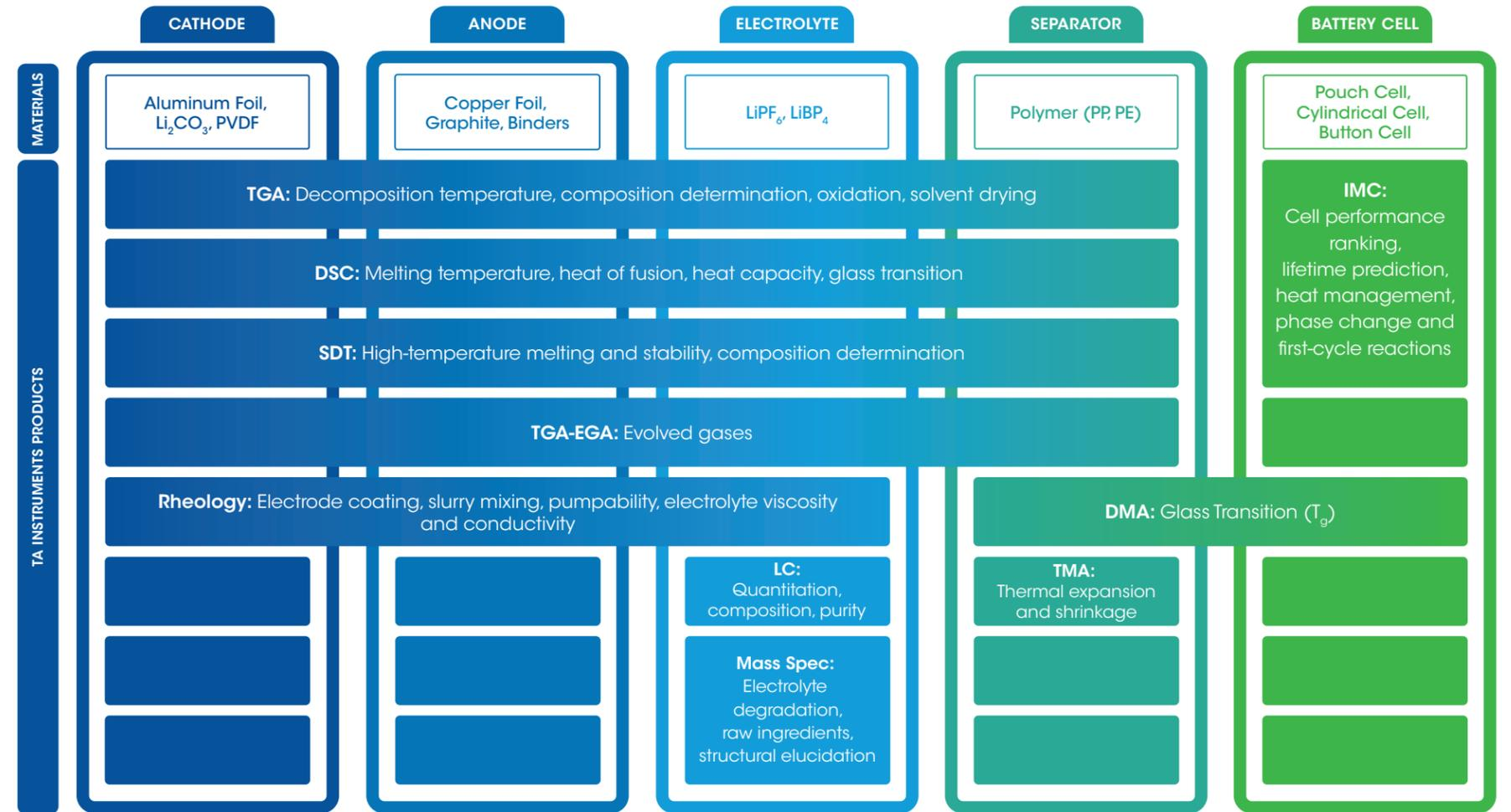
**Table 2.** Parameter insights provided by material characterization techniques of the four main components of a lithium-ion battery and the whole cell.
