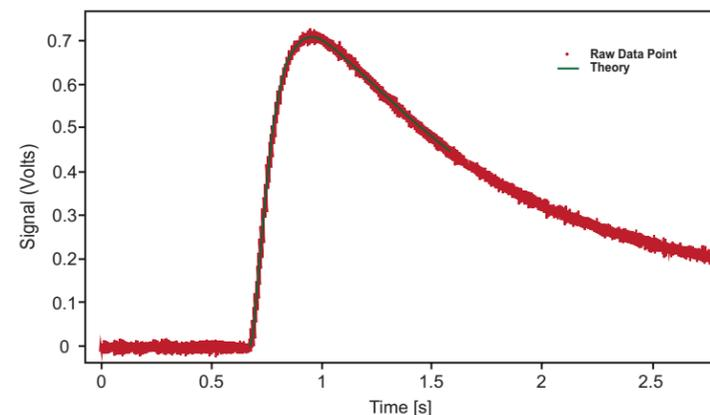
**Figure 9.** Thermogram of the copper thin film (red) fitted with Fin theoretical model (green) in excellent agreement. The thermal diffusivity was determined as 1.17  $\text{cm}^2/\text{s}$ .
