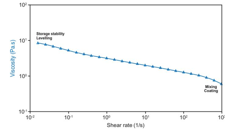
Figure 8. Viscosity vs shear rate of an LIB electrode slurry over 5 decades of shear rates. The slurry exhibits shear-thinning behavior with the viscosity decreasing with increasing shear rate.
