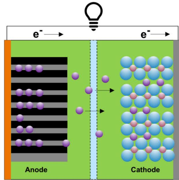
**Figure 1.** Schematic of a lithium-ion battery. The four main parts of a lithium-ion battery are the cathode, anode, electrolyte, and separator.
