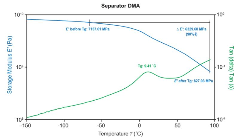
Figure 6. DMA of separator film in x-direction. Note the glass transition,  $T_g$ , at 9.41 °C (green curve) and a 90% drop in  $E'$  (blue curve) as the material undergoes a glass transition.
