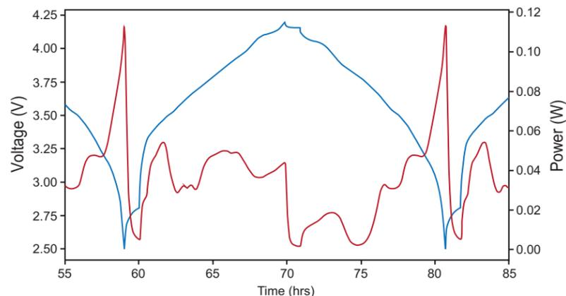
**Figure 10.** Raw data of voltage (blue) and power (red), versus time for an 18650-battery cell, cycled at C/10 in the TAM IV isothermal microcalorimeter.
