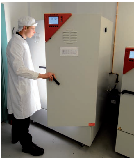
▲ KBF P constant climate chamber in use
