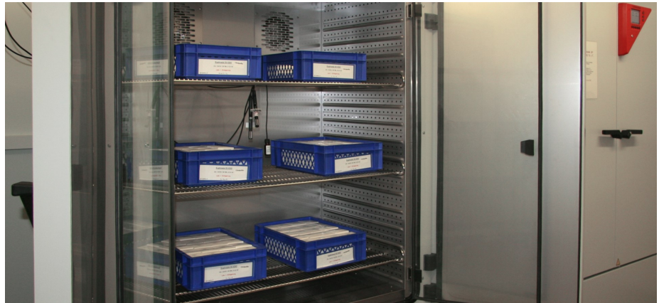
▲ Medicine stability test in a KMF constant climate chamber
